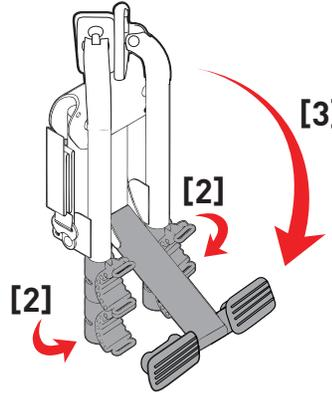
4. ROTATE BOTH TOP FEET DOWN BY 90 DEGREES TO OPEN, FULLY ENGAGING PINS
