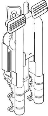
2. ROTATE TIE-DOWNS, AND FULLY EXTEND BOTTOM FOOT
